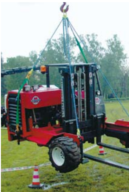
Lifting with GrabIQ sling.
