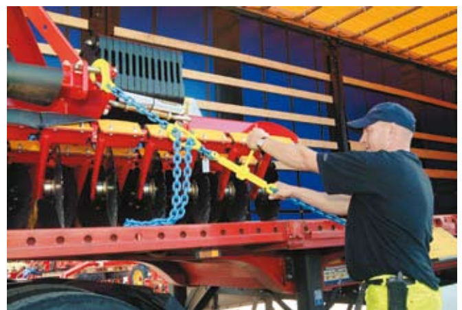
Cargo securing of agricultural equipment.
